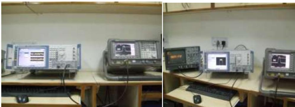
**Vector Signal generator and Spectrum Analyser**
