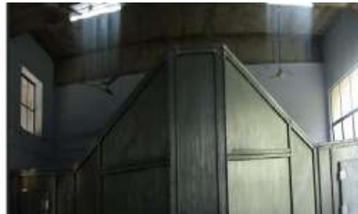
**Anechoic chamber for antenna testing**
